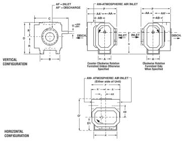
Drive shaft Approx net Wt. (lbs) Frame Size location С 0 0' ΑВ AF в Р Р R U AA AA' AF AW АΧ Keyway 12 14 12 827J 19.00 27.00 33.18 46.54 18.00 10.00 26.50 25.75 25.25 25.25 14.00 2.625 .625 x .313 9.50 15.25 5.50 4.00 2100 FLG FLG FLG
