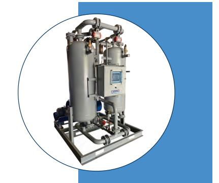
In a twin tower desiccant air dryer, one tower is on-line drying the compressed air while the other is off-line regenerating, which means it is eliminating the water vapor it has collected so it can be used to dry again. The two towers switch back and forth so one is always drying while the other is regenerating or in standby.
